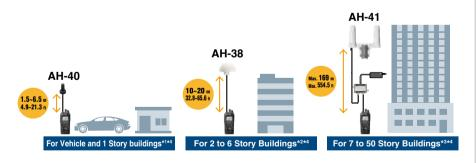
\*1 Optional OPC-2422 coaxial cable (5 m, 16.4 ft) is required for more than 1.5 m, 4.9 ft extension.
