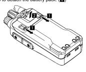
Lift the tab up (1), and slide the belt clip in the direction of the arrow (2). Detaching:
