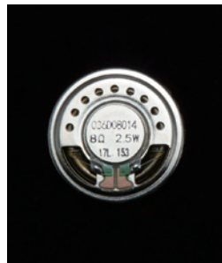
Icom custom high power handling capacity speaker
