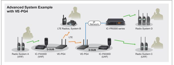
The VE-PG4 is a versatile RoIP (Radio over IP network) gateway unit, which interconnects the IC-F5330D series with other radio systems, even when the systems are using different bands\*.
