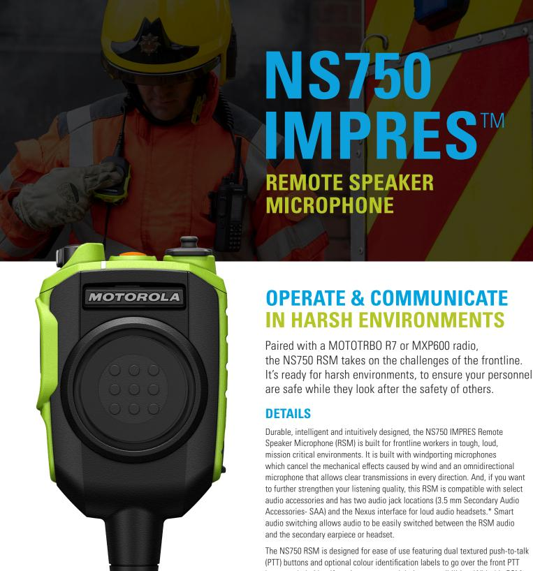
audio accessories and has two audio jack locations (3.5 mm Secondary Audio Accessories- SAA) and the Nexus interface for loud audio headsets.\* Smart audio switching allows audio to be easily switched between the RSM audio The NS750 RSM is designed for ease of use featuring dual textured push-to-talk
