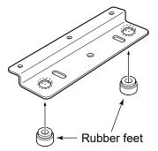
2. Attach the mounting plates to the Main unit using the 6 supplied hex head bolts (6 × 15 mm), 6 flat and spring washers, as shown below.
