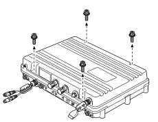
2. Open the Main unit, and then disconnect 1 flat and 2 coaxial cables, as shown below.
