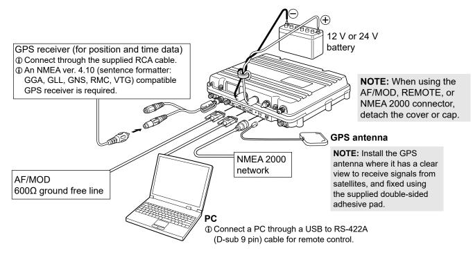
**CAUTION:** When an external unit is connected, such as a PC, it must be properly grounded. (p. 61)
