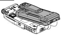
☐ To remove the battery, turn the radio off. Slide the Battery Pack Latch on the bottom of the radio, then lift up on the bottom of the battery and remove it from the radio.
