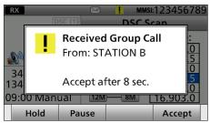
[Hold] Puts the RX task on hold and returns to the Main screen.
