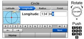
① Displays your vessel's position data as the default. ① To select 'W' (West longitude) or 'E' (East longitude), select "W" or "E" on the screen and push [ENT], or push a Keypad key when the cursor is on the 'W' or 'E.'
