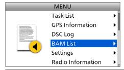
**TIP:** You can also enter the BAM List screen by holding down [CH/ENT] for 1 second on the Main screen.
