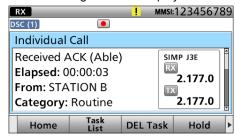
• When the BAM function (p. 18) is OFF: The backlight blinks and the popup screen is displayed. Push [Alarm Off] \_\_\_\_, and then push [Close Call RCVD Window]
