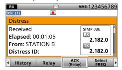
6. Push [Call] to send the Distress Relay Acknowledgment.
