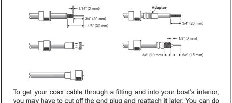
you may have to cut off the end plug and reattach it later. You can do this if you follow the directions that come with the connector. Be sure to make good soldered connections.
