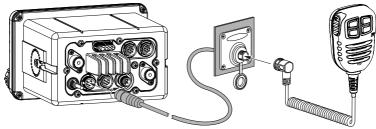
In addition, the **GX6000E** is capable of connecting hand microphone to the connector on either the front or rear panels.
