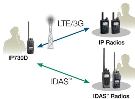
Communication redundancy, when network congestion occurs or network service is temporarily unavailable
