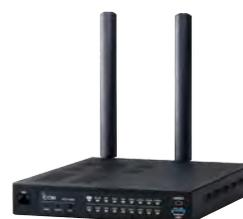
With a VE-PG4 RoIP gateway, the IC-SAT100/M can interconnect with an IP phone, IP, WLAN, IDAS™ digital (Type-D multi-site trunking and conventional systems.) and analog transceivers.
