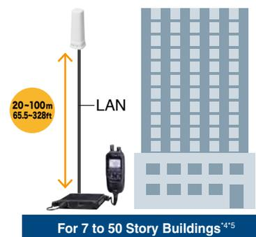
\*<sup>1</sup> Optional OPC-2422 coaxial cable (5 m, 16.4 ft) is required for more than 1.5 m, 4.9 ft extension.
