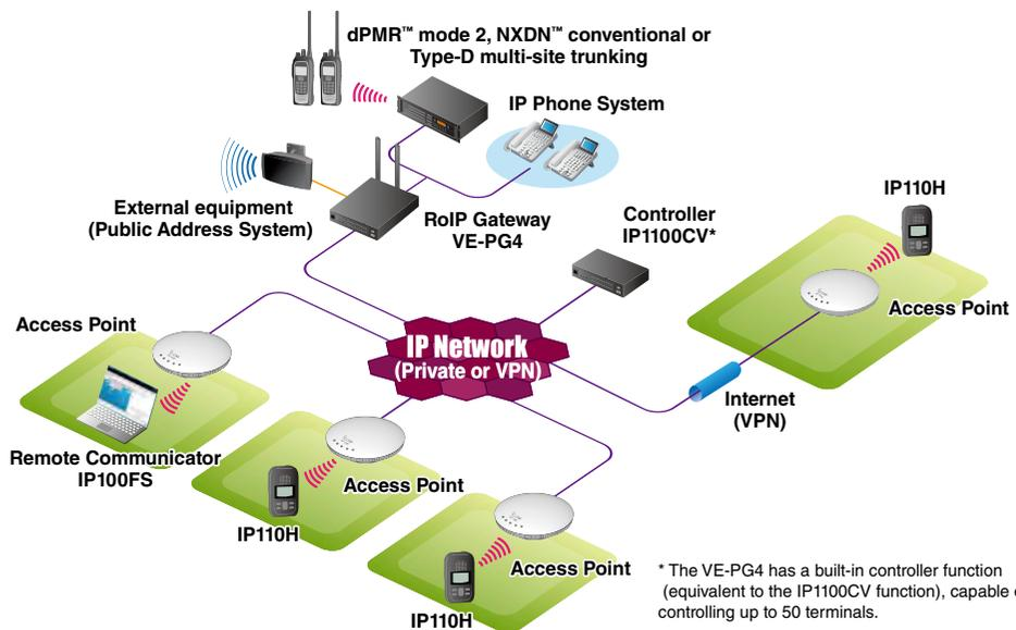
\* The VE-PG4 has a built-in controller function (equivalent to the IP1100CV function), capable of controlling up to 50 terminals. The figures leave out some equipment, such as a network switch, to simplify the information.
