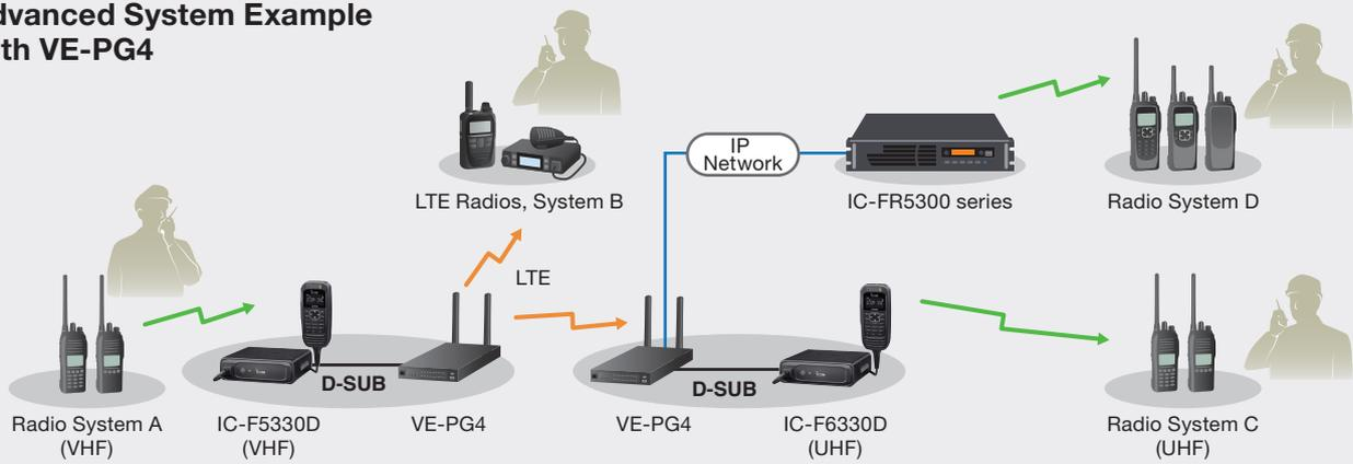
The VE-PG4 is a versatile RoIP (Radio over IP network) gateway unit, which interconnects the IC-F5330D series with other radio systems, even when the systems are using different bands\*.
