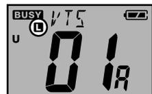
4. If using Low power is not effective, select High power (5 watts: “**H**” icon disappears) by pressing the
