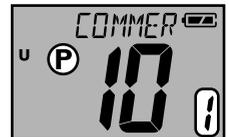
3. To exit from the Preset channel mode, press the
