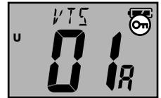
2. Hold down the
