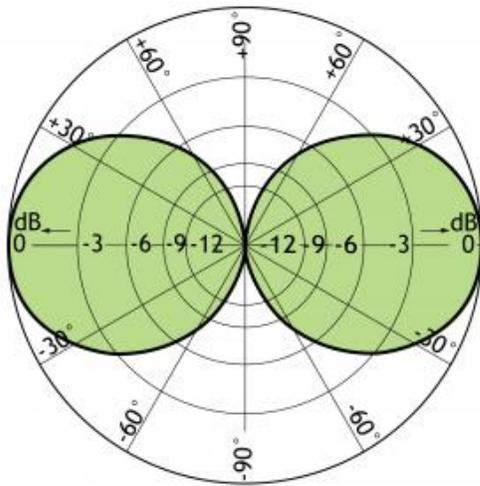
TYPISCHES STRAHLUNGSDIAGRAMM (HORIZONTAL)
